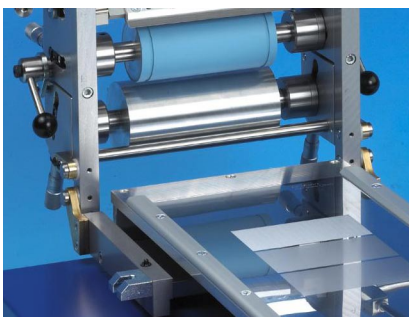
▲ Detail of K Printing Proofer Flexo Head
